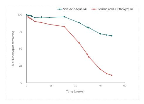
Large scale trial: 1000 litre containers stored outside exposed to all kinds of weather conditions. Sampling started in October 2010. The results are measured by HPLC. Note: Slow degradation of ethoxyquin during winter period due to very cold weather. Laboratory trials have also been performed (at 20-25°C), supporting the above mentioned results. The stability trials all show that lignosulphic acid has a stabilising effect upon ethoxyquin.
