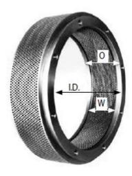
Die working area is defined as the area between the two inside die grooves. This working area increases as die width and diameter increase. Die working area is important because different feeds and ingredients require specific amounts of time in the die hole—die retention time—to be able to bind together to form a pellet. Larger die working areas provide more retention time to form pellets, reduce power consumption per tonne of feed pelleted and improve production efficiencies.
